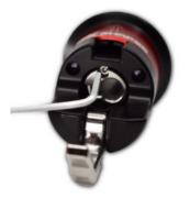
Loosen the two screws on the bottom plate spinner with a 2mm hex key.
