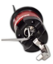
Place the assembled bottom plate spinner into the cavity and tighten the screws (torque: 0.5Nm - finger tight).
