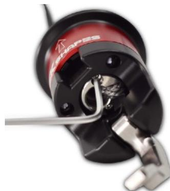
Place the assembled bottom plate spinner into the cavity and tighten the screws (torque: 0.5Nm - finger tight).
